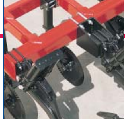
Shank-Stagger Kit for increased residue flow
