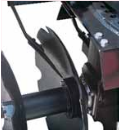
Blade scraper kit/triple-lip sealed bearings
